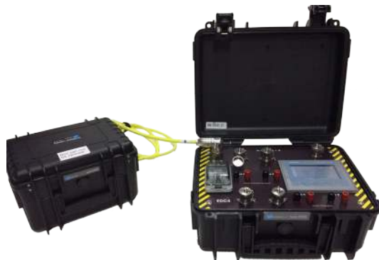
Control unit and 24V transformer/opt accumulator
